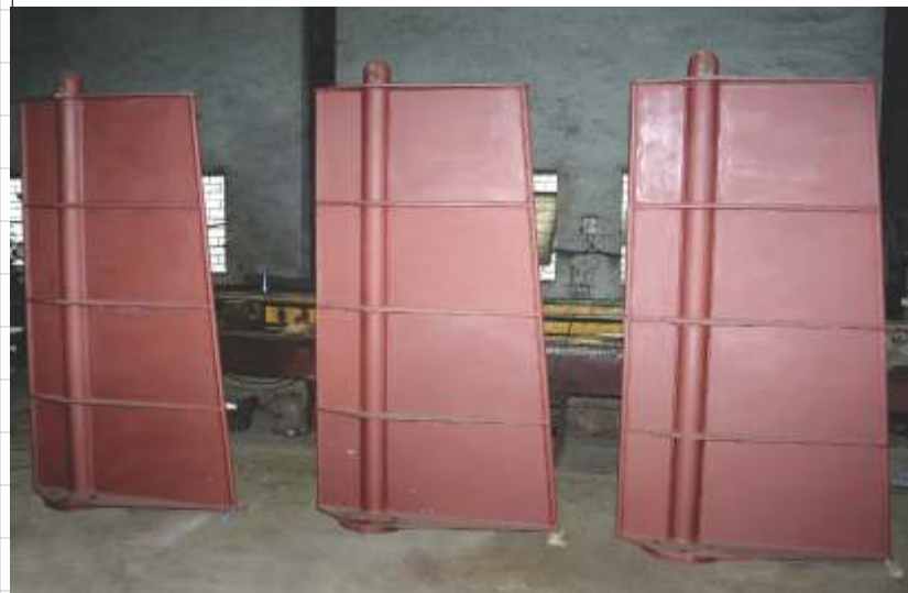
◀ Rudder Stock Arrangements for Tug Boats
